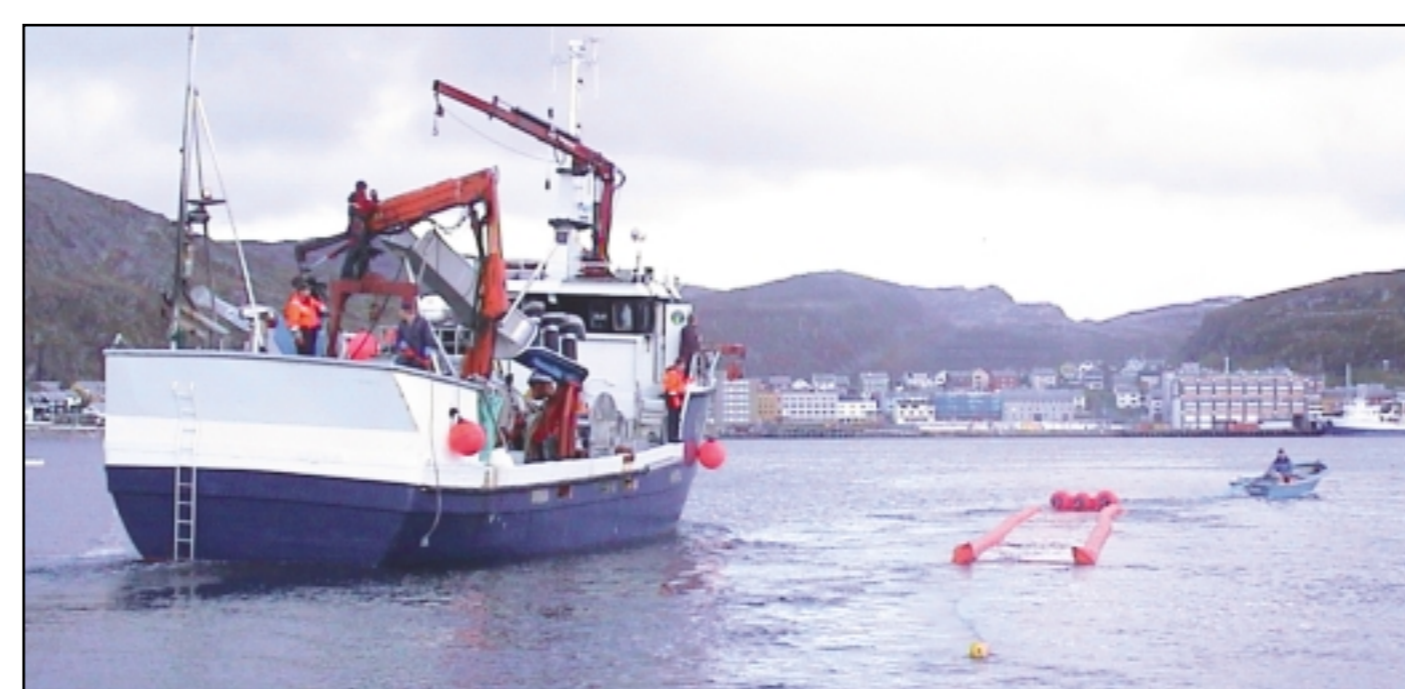
The towing cylinder is set afloat over the stern. It can be towed and kept open by the coastal seiner's life-boat, and is taken on board through the triplex.
