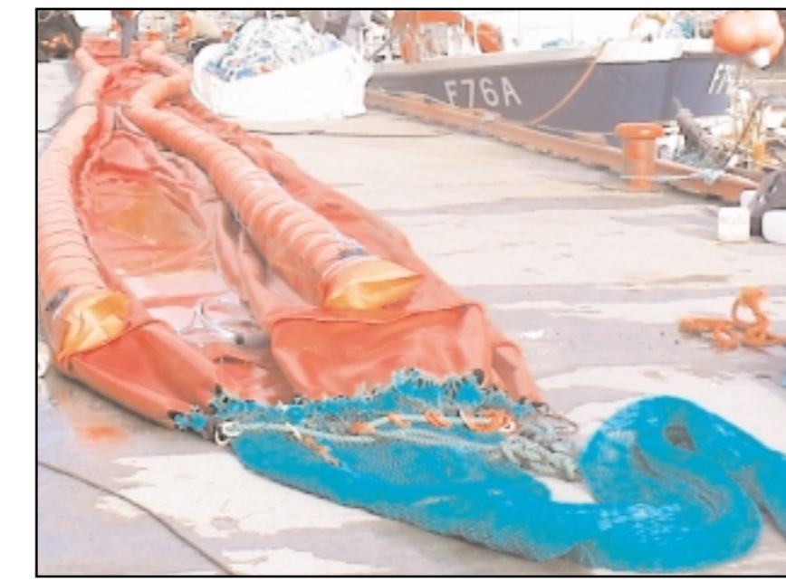
Assembling net, floaters and ropes at the jetty.
